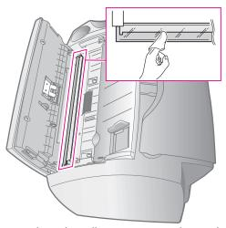
6. Replace the roller in reverse order, and then close the control panel firmly until it clicks into place.
